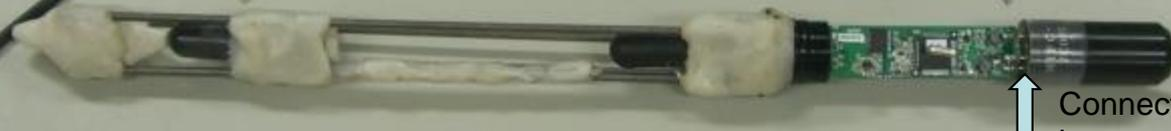
Connect here. Same manner as the battery box as shown below (there are five outside pins for power supply. Inside pins are for communication).
