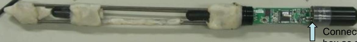
Connect here. Same manner as the battery box as shown below (there are five outside pins for power supply. Inside pins are for communication).
