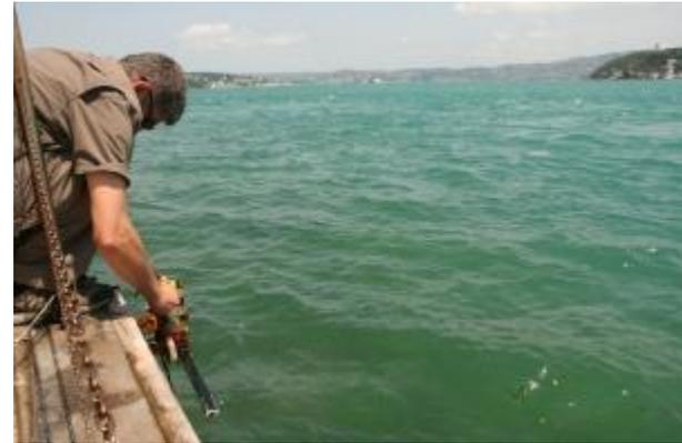
**Attendance and swimming directions could be measured using stationed A-tag on a seabed or a buoy.**
