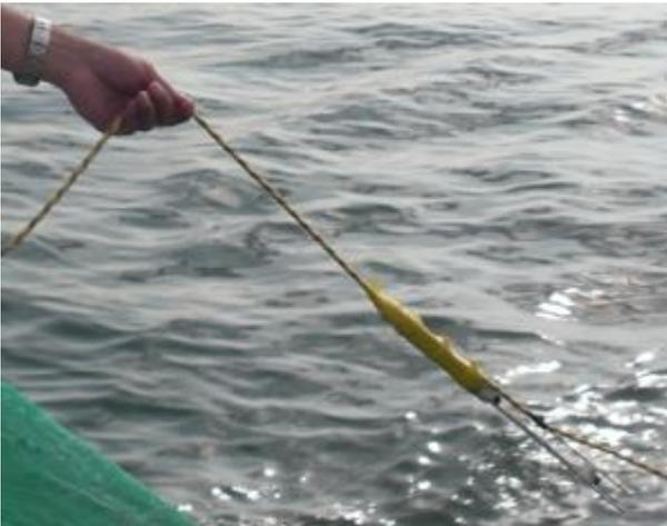
*A-tag* fixed on a rope towed from a boat (left).
