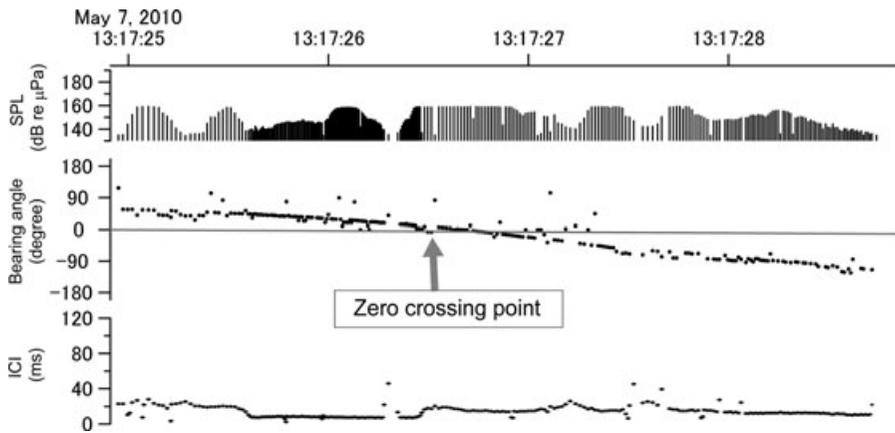
Figure 2. An example of echolocation signals from a single porpoise passing the data logger. Vertical axes show the received SPL (dB re 1  $\mu$ Pa), bearing angle (degree), and interclick intervals (ICI; ms). The bearing angle tracks from positive to negative, indicating that an echolocating porpoise passed from bow to stern of the towed A-tag.
