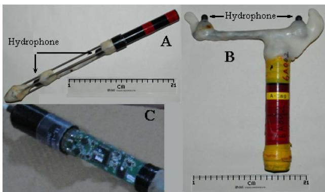
FIG. 2. (Color online) External and internal appearance of the miniature stereo acoustic event data-logger (A-tag). (a) External appearance of a linear type A-tag with one CR2 lithium battery inside used for relatively short-term acoustic survey; (b) external appearance of T-type A-tag with two alkaline UM-1 batteries inside used for long-term acoustic survey up to one month; (c) internal appearance of a A-tag with electronics module containing.
