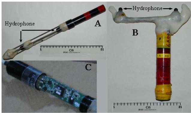
FIG. 2. (Color online) External and internal appearance of the miniature stereo acoustic event data-logger (A-tag). (a) External appearance of a linear type A-tag with one CR2 lithium battery inside used for relatively short-term acoustic survey; (b) external appearance of T-type A-tag with two alkaline UM-1 batteries inside used for long-term acoustic survey up to one month; (c) internal appearance of an A-tag with electronics module containing.
