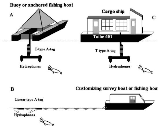
FIG. 4. Diagrams of the passive acoustic monitoring and detection platforms. (a) A buoy or anchored fishing boat for fixed passive acoustic monitoring deploying a T-type A-tag; (b) a customizing survey boat or fishing boat towing two linear type A-tags for passive acoustic surveys in joint visual-acoustic surveys or regular fishing boat based long-term passive acoustic surveys; (c) cargo ship based survey platform deploying a T-type A-tag.
