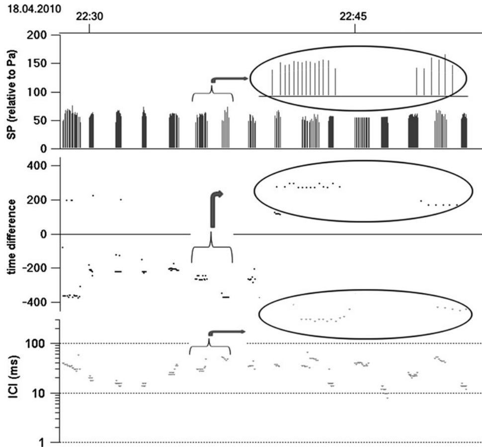
Fig. 3. Click trains recorded by A-tag: top, sound pressure; middle, time difference of sound arrival; bottom, inter-click interval.
